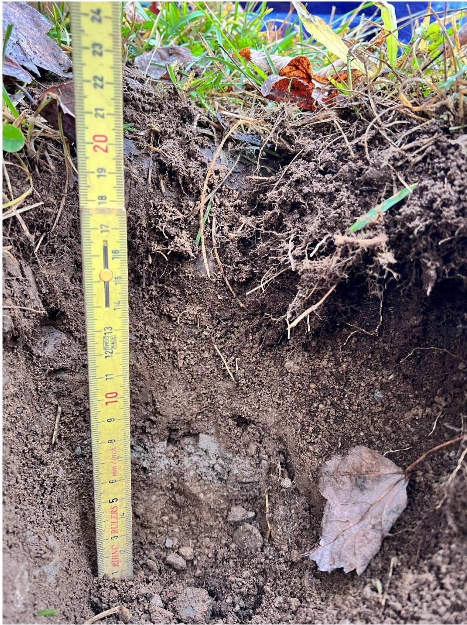
Figure 9: Shovel Test #12, A Horizon, B Horizon, and a B Horizon with gravel (11/14/25)
