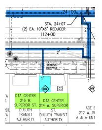
• 1" Logstor Integrated Twin Pipe System entering building from Superior St.
