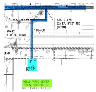
• 3" Logstor Integrated Pipe System entering building from Superior St.
