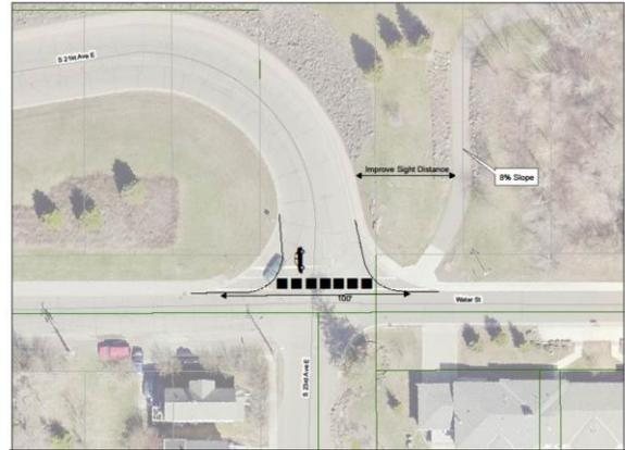
Intersection Concept by the City of Duluth Engineer with a more visible crosswalk and smaller corner radii.
