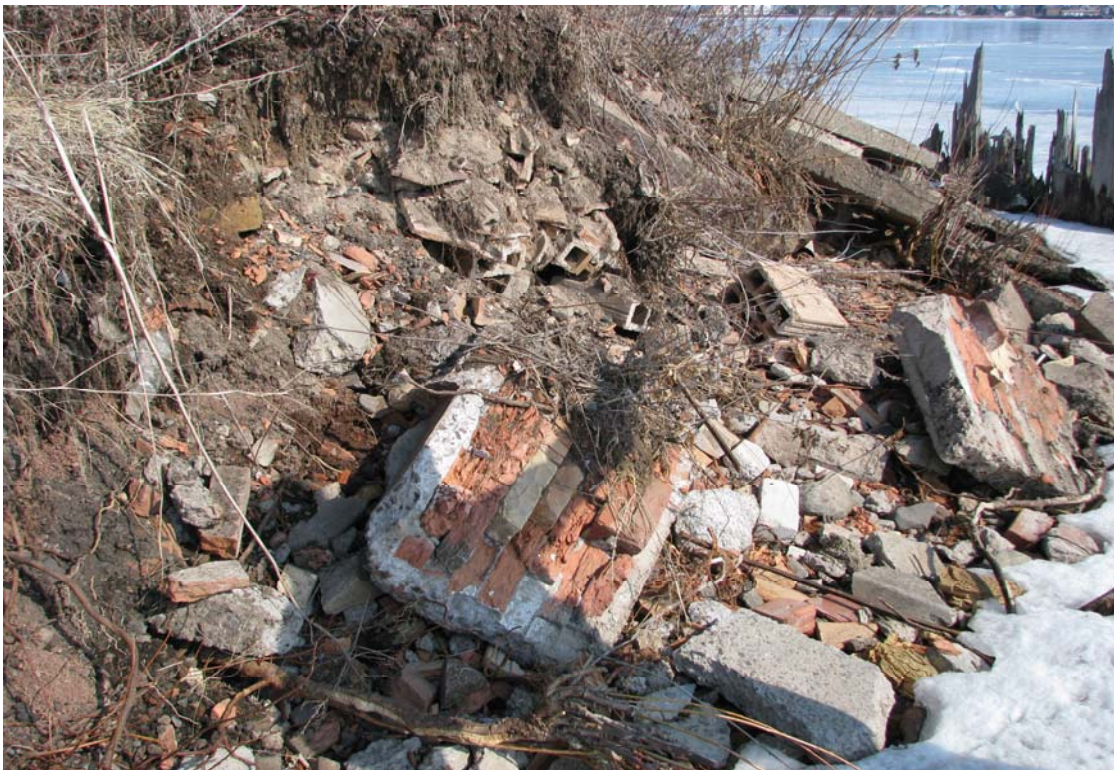
Photo 24 Close-up of fill with abundant bricks, mortar, cement and soil at eroded southeastern side of Lot D area. Harbor in background.
