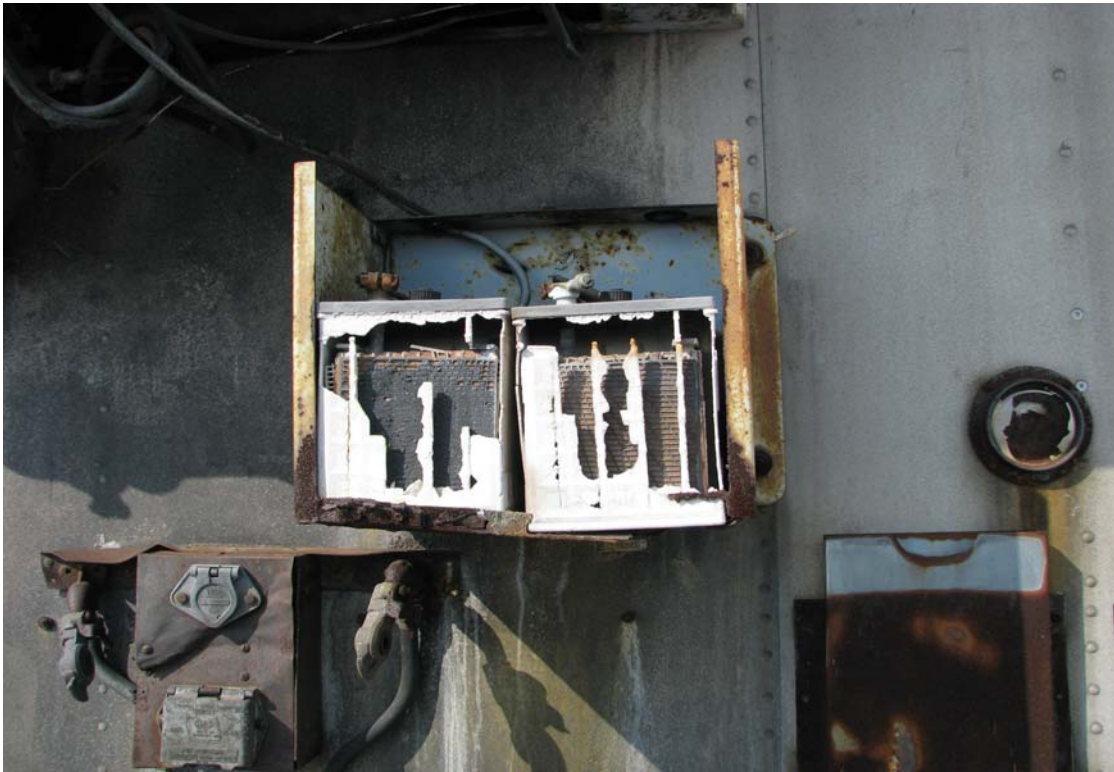
Photo 13 Close-up of deteriorating batteries on end of left semi trailer.
