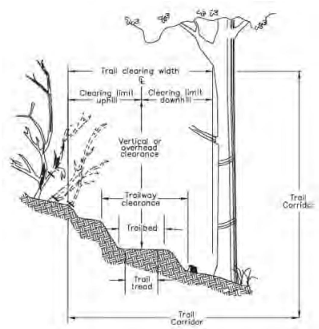
Figure 4: Clearing limits
