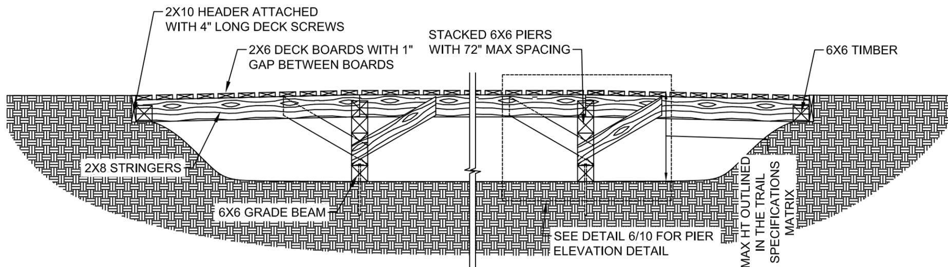
**TYPICAL ELEVATION DETAIL FOR BOARDWALK (WET AREA CROSSINGS)**
