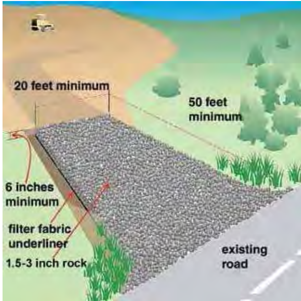
Rock Construction Entrance
