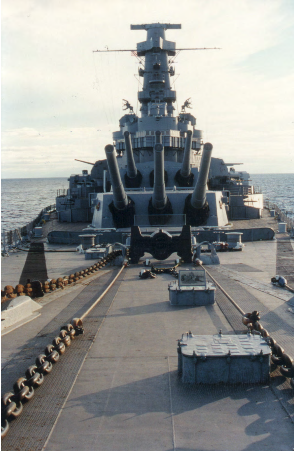
Both legs of towing bridle inboard can be seen on foredeck with wire shackled to towing eyes and chain bridle.
