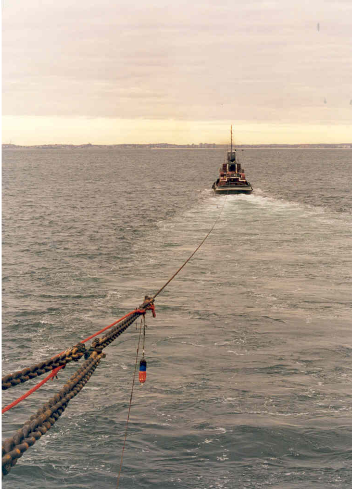
Excellent view of tow chain bridle and retrieval lines as tug 'ESTER MORAN' commences shortening wire entering Boston Harbor.
