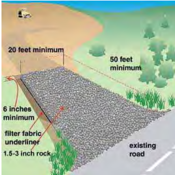
Rock Construction Entrance
