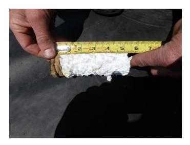
A core sample reveals EPS and wood fiber layers – no moisture was identified within the substrates.
