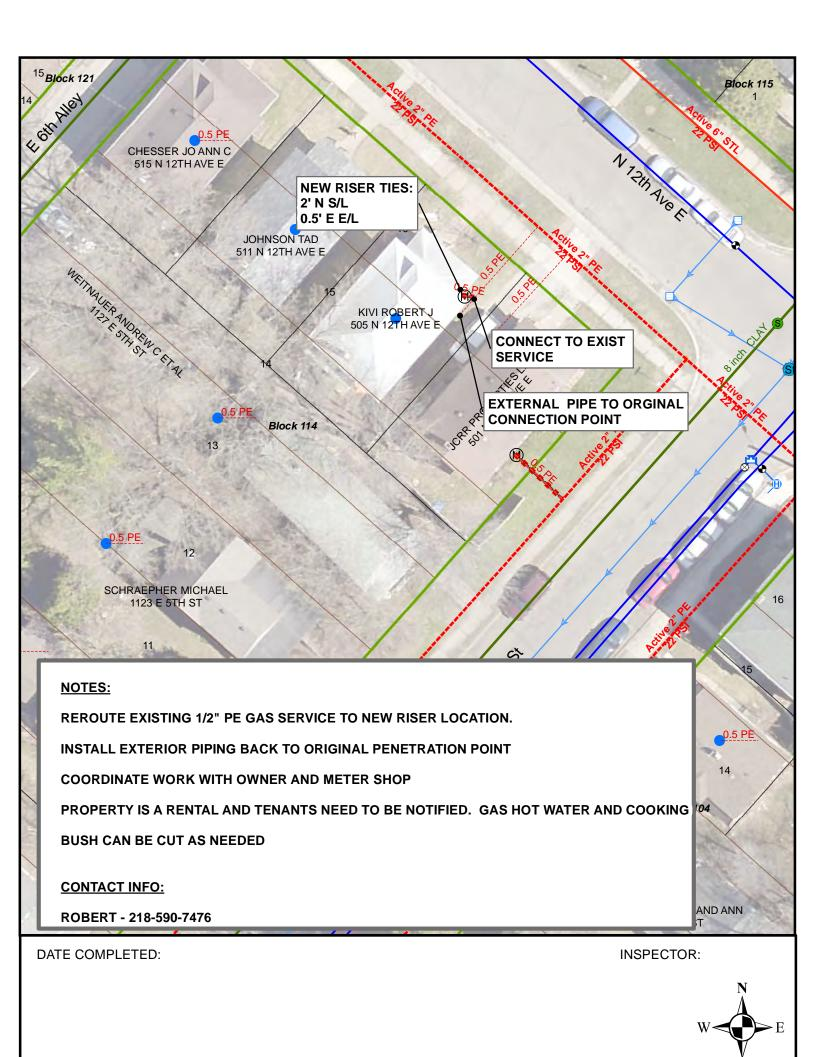
EAM #: 430894 ZONE: 4 EXCESS FLOW VALVE: NA APPL#: NA REROUTE EXISTING 1/2" PE GAS SERVICE PLAN OF: \_\_ LOCATION: 505 N 12TH AVE E FROM: TO:
