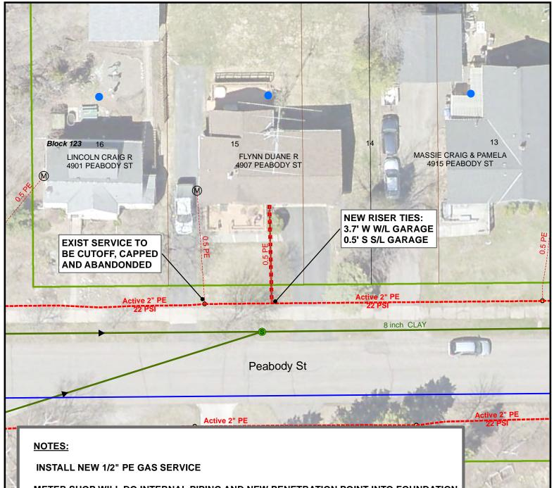
METER SHOP WILL DO INTERNAL PIPING AND NEW PENETRATION POINT INTO FOUNDATION.
