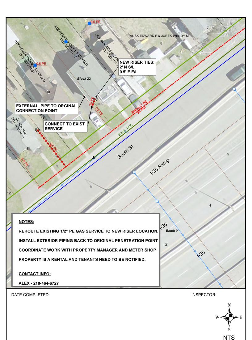
EXCESS FLOW VALVE: NA APPL#: NA EAM #: 430894 ZONE: 4 REROUTE EXISTING 1/2" PE GAS SERVICE PLAN OF: \_\_\_
