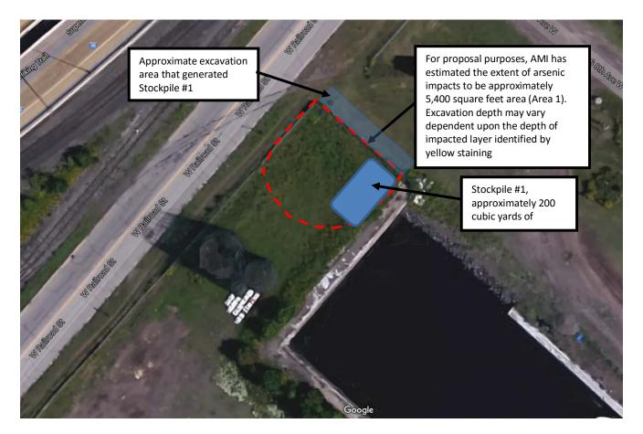
Step 1 – Load, Transport and Dispose of Stockpile #1 which is already created. Stockpile #1 is estimated to be approximately 200 cubic yards and is currently located at the head of Slip 3. This soil has been tentatively
