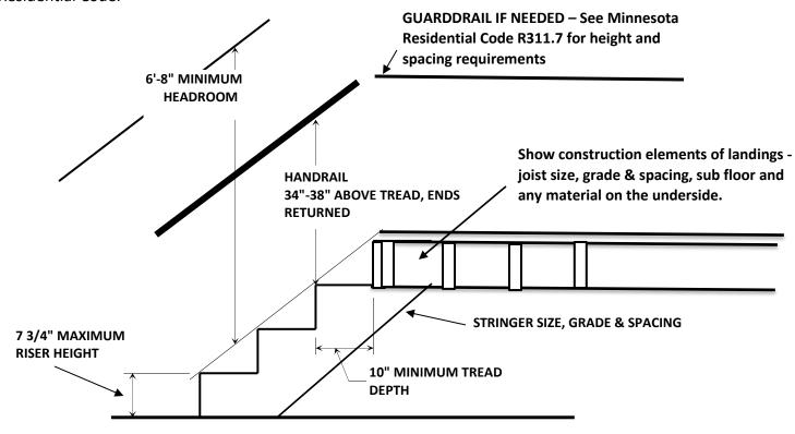
**Landings for stairways**. There shall be a floor or landing at the top and bottom of each stairway, except at the top of an interior flight of stairs, provided a door does not swing over the stairs.
