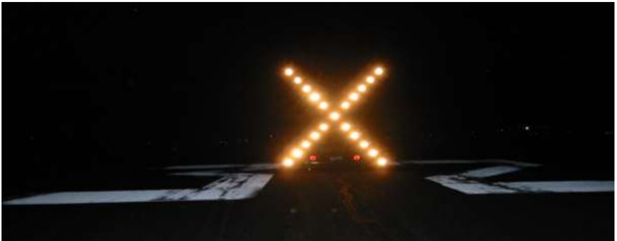
Figure 2-4 Lighted X at Night
