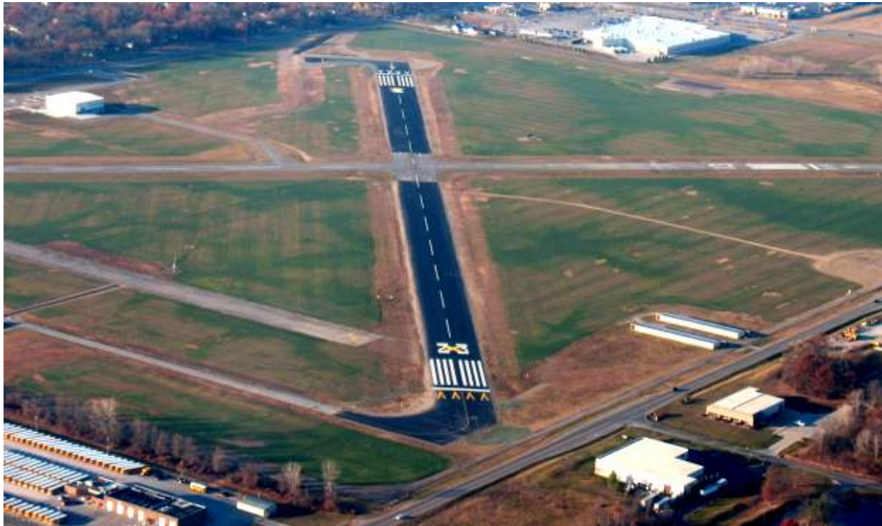
Figure 2-1 Markings for a Temporarily Closed Runway
