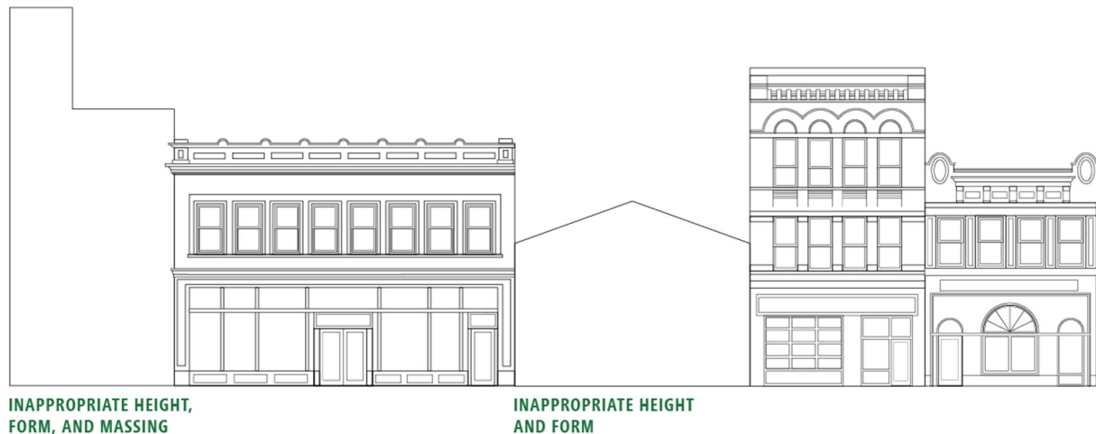
Figure 9: Diagram showing the effect of inappropriate infill. The infill in the upper streetscape is inappropriate in height, scale, and style, and disrupts the rhythm and unity of the block.
