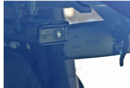
**Rear Squad Cameras:** All squad cars have a camera that begins recording once an individual is being transported, or the back doors of the squad car are open.
