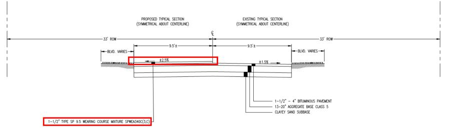
W. 6TH ST. - 466 FEET E. OF 8TH AVE. W. TO 932 FEET E. OF 8TH AVE. W. IN-PLACE TYPICAL SECTION APPLIES: STA. 00+99.00 TO 06+55.00
