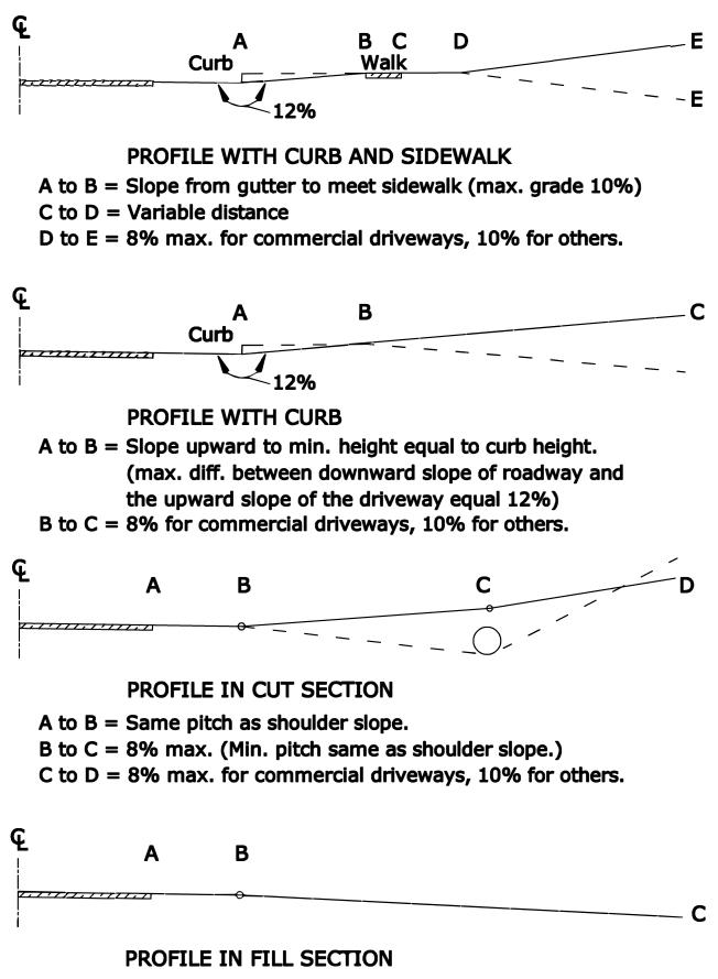
A to B = Same pitch as shoulder slope. B to C = 8% max. for commercial driveways, 10% for others.
