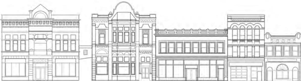
*Figure 8: Diagram showing the typical unity, scale, and massing within the Duluth Commercial Historic District.*
