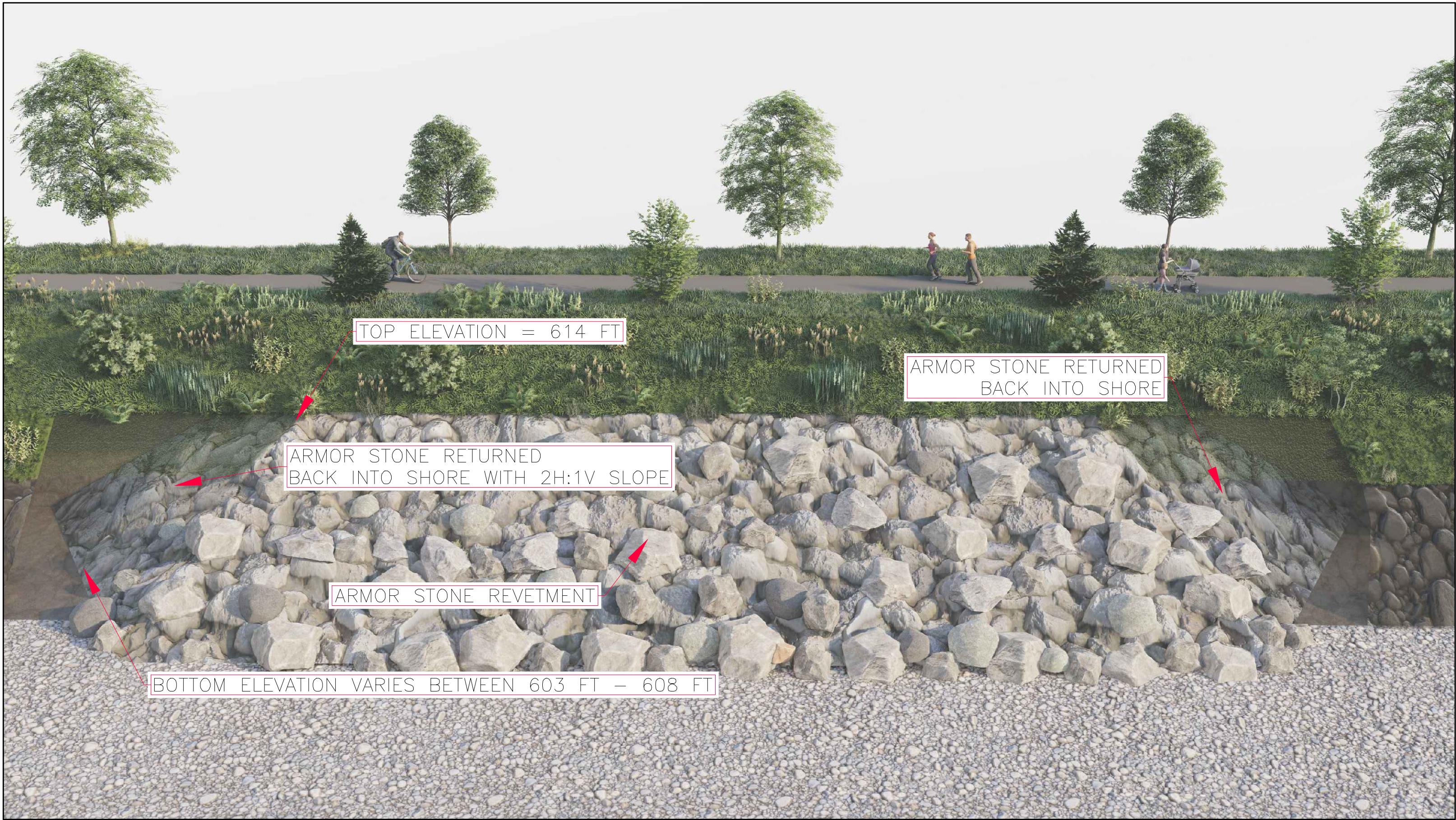
2 C2.9.1 REVETMENT RETURN DETAIL
