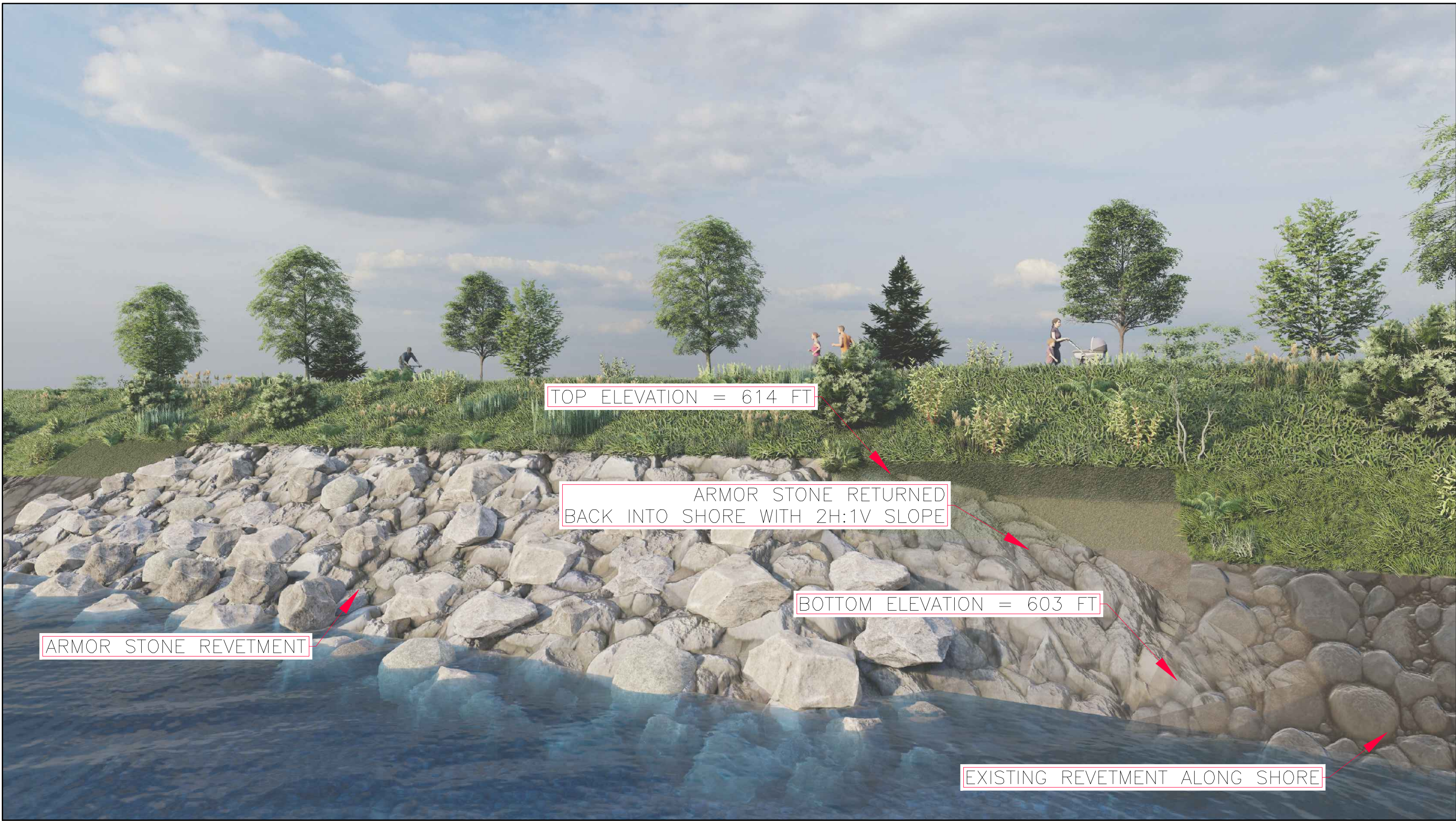
1 C2.9.1 TYPICAL REVETMENT RETURN DETAIL
