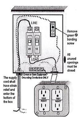
The disconnect may be permanently installed within a concession stand or mounted to a portable backboard.
