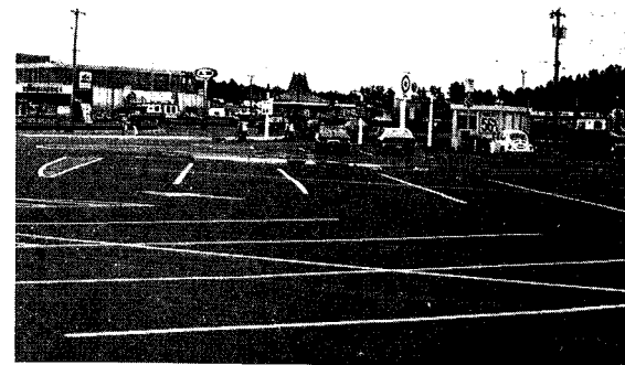
The addition of impervious surfaces greatly increases the concentration of stormwater runoff.
