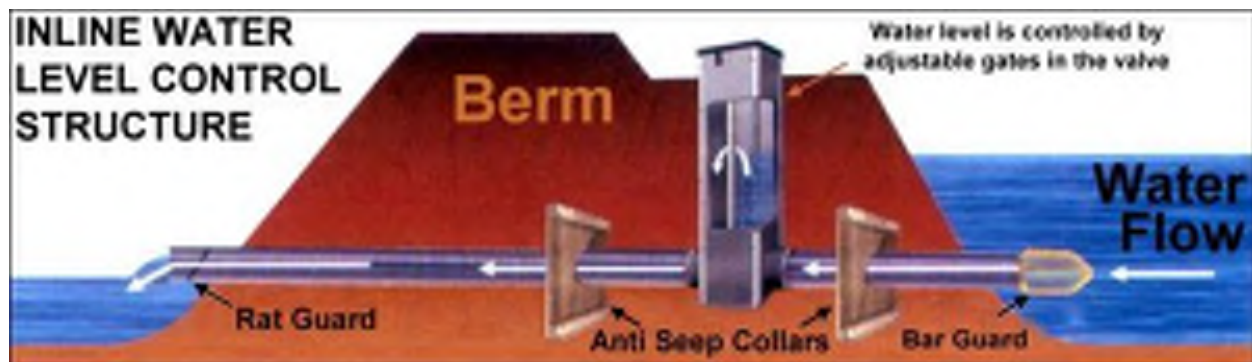
Figure 8: Conceptual image of a bottom withdrawal structure (Keppler, 2011).
