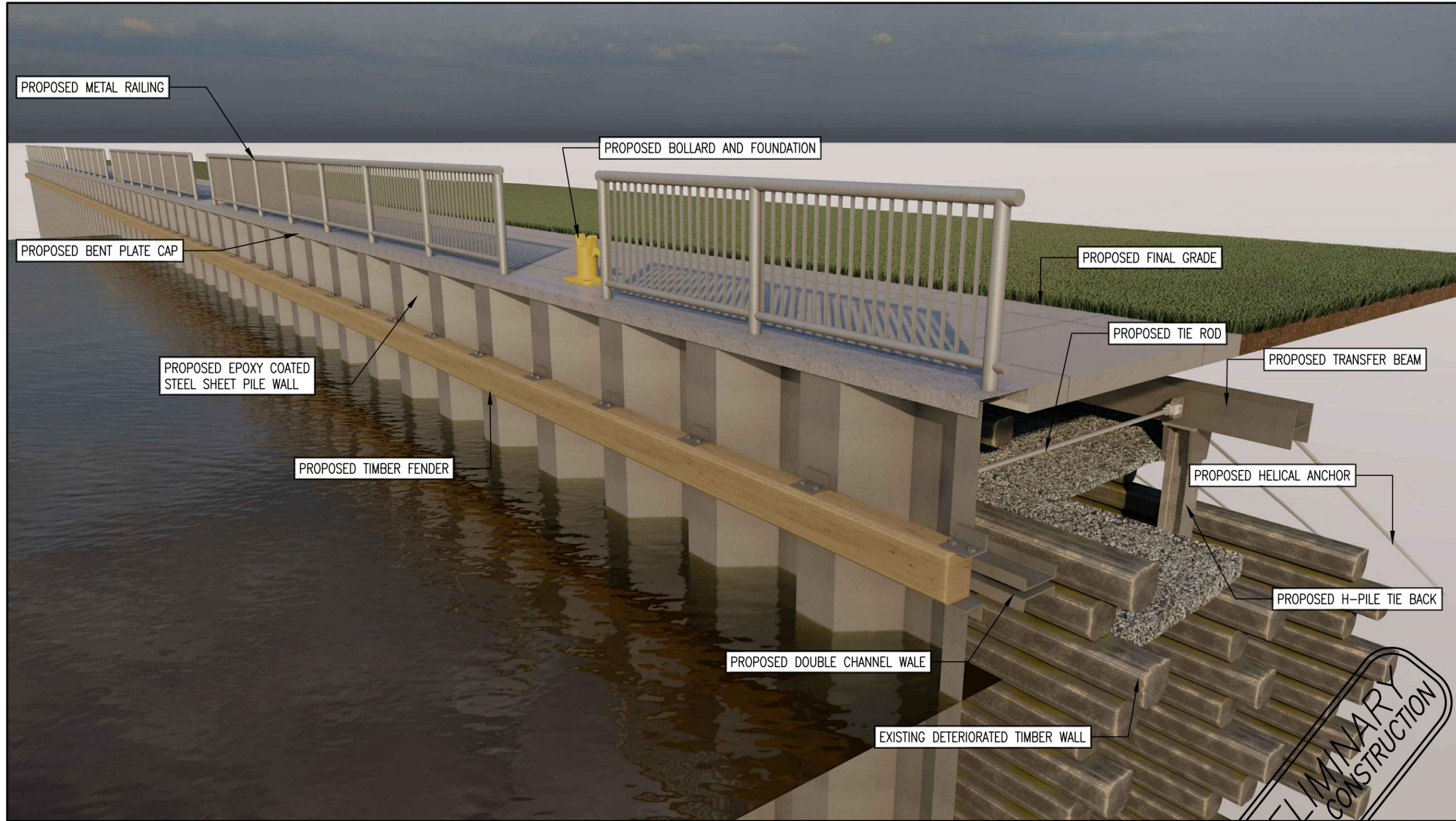
1 DECC SEAWALL - PROPOSED TIMBER CRIB REHAB RENDERING
