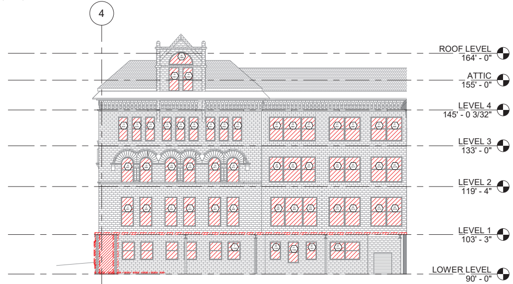
3 DEMO - EAST DOCK - NORTH ELEVATION D10.2 1/16" = 1'-0"
