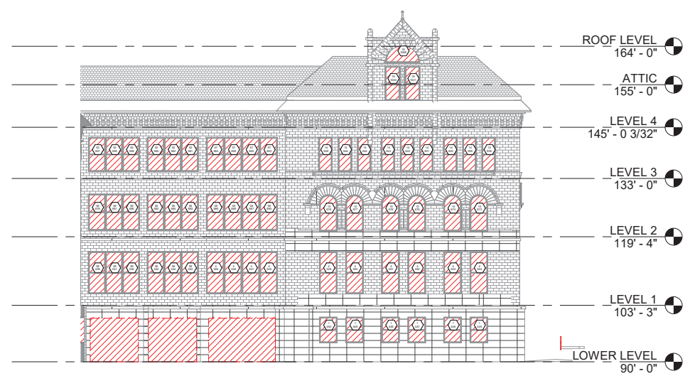
2 DEMO - WEST DOCK - NORTH ELEVATION D10.2 1/16" = 1'-0"
