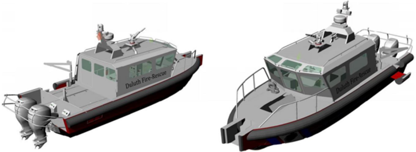
Conceptual drawing of a 31' X 10.5' All Hazard Quick Response Vessel
