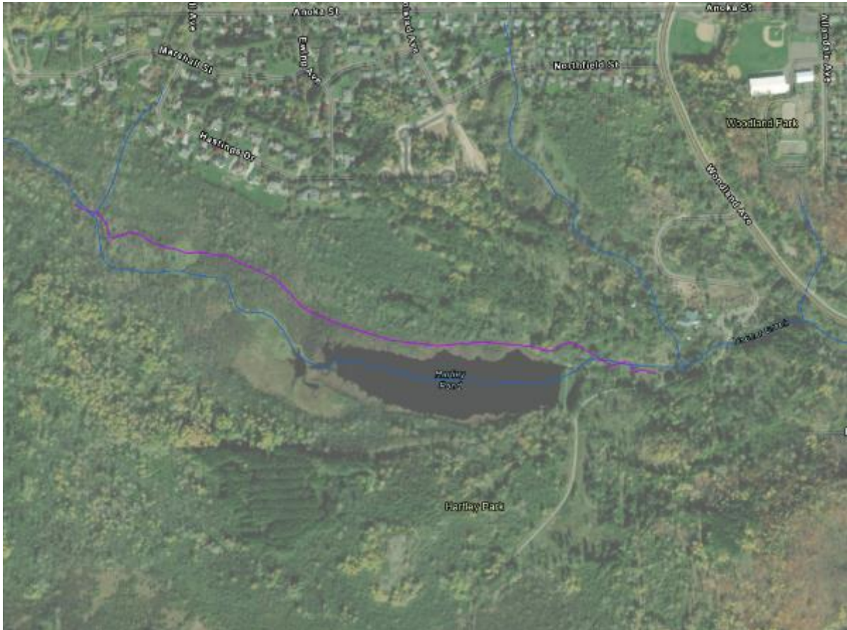
Figure 19. Modeled Tischer Creek channel re-route (purple) in relation to current stream channel (blue).
