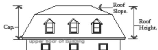
Pitched Roof cap type - Mansard
